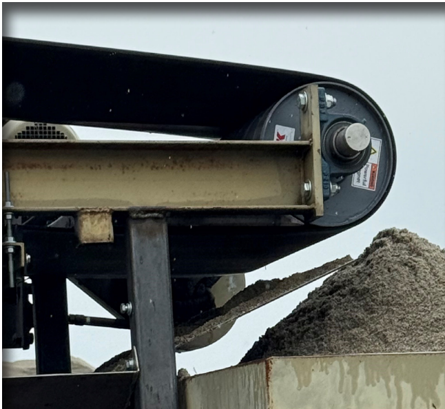
Photo: K-Magnetic Separator Pulley installed at the head drum.
