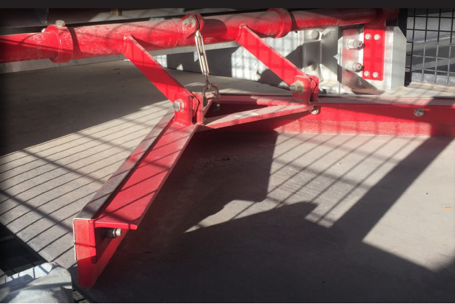
K-Safeguard Vee Plough Belt Cleaner helps clear debris.
