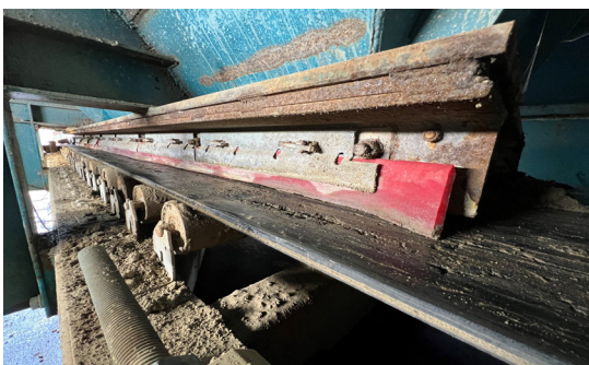
Before Photo: Cheap & inferior poly skirting was unable to withstand the pressure.
