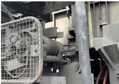
The operator previously used standard H-Type Tungsten and High Temperature Resistant Polyurethane blades with a temperature resistance of up to 150°C. Due to the high temperature environment, the Tungsten H-Type belt cleaners conducted the ambient heat from the furnace and subsequently damaged the conveyor belt.
