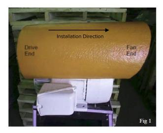
Covers arrive without a cut-out for the conduit box or lifting lugs (if there are any). After making sure that the motor cooling fin channels and air intake are clean, install the cover by aligning the back end so that they are fully covered. Fig. 1
