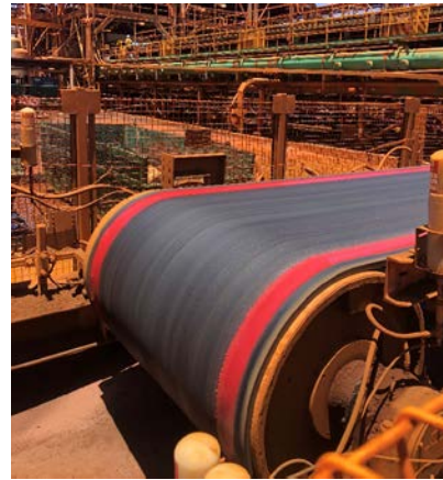
Figure 4 - Belt cover repair system shown here to fill in grooves caused at skirt zones (Wear Systems Solutions)
