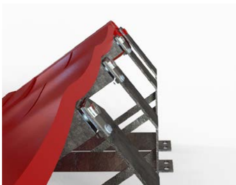
Figure 13 - Possible failure mode under high ambient temperature or high belt speed and capacity conditions, placing higher loads on smaller areas due to sagged slider rails once the softening temperature is reached
