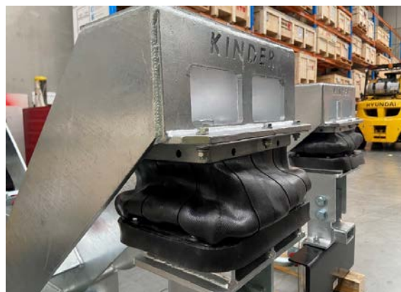
Figure 12 - Torsion spring boot added to prevent ingress
