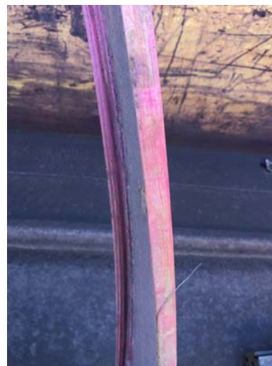
Figure 6 - Variable wear thickness along slider rail
