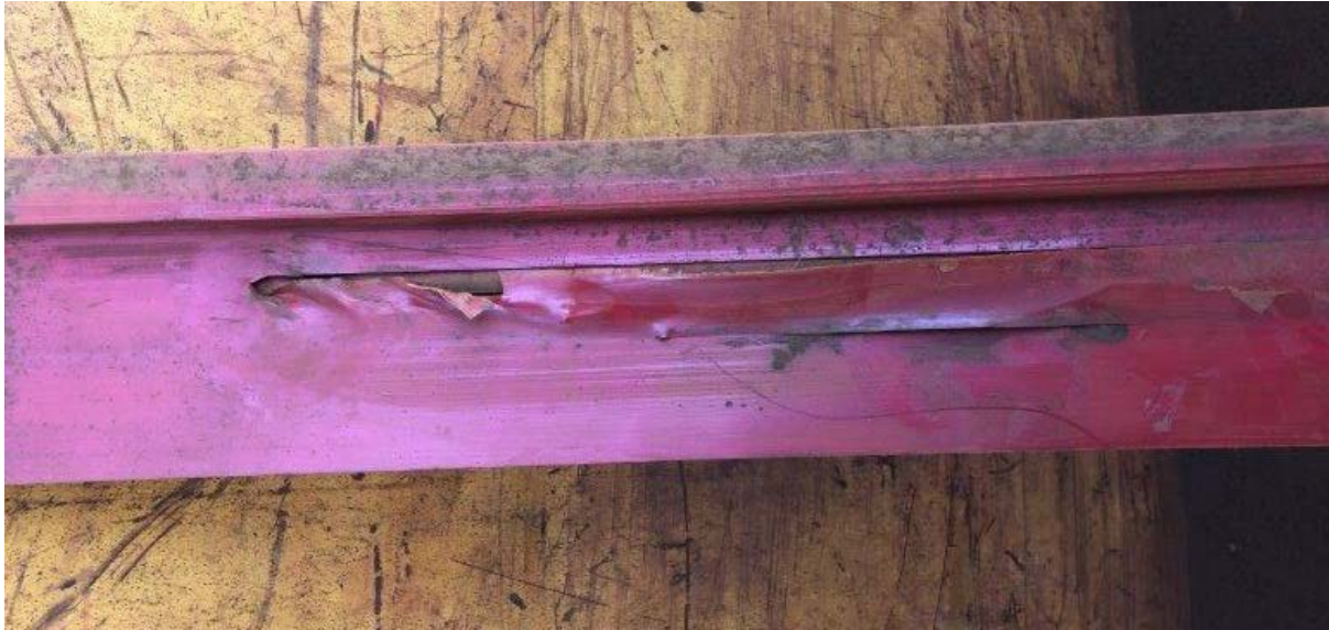
Figure 15 - Signs of friction generated burning on the slider rail
