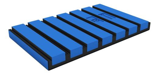
Elastotec Polyurethane Lagging is 250mm wide to ensure easy handling and application. It is supplied in long roll lengths that fit on standard sized pallets to eliminate waste and for cost effective transportation and storage. It can be supplied in thicknesses from 10mm to 20mm.
