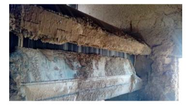
Antofagasta Minerals Antucoya operation had been experiencing low wear life of their primary belt cleaner blades installed within their reclaiming conveyor system, which has a throughput of 9.000 tph, mostly using conveyors with 1829mm wide belts at 6.2 m/s.
