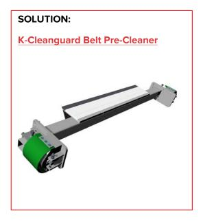
We recommended installing K-Cleanguard Belt Pre-Cleaners at the discharge of every conveyor, focused on separating the main ore flow of the conveyor belt and extending the wear life of the primary belt cleaner's blade. A special pre-cleaner wear plate had to be designed for Antucoya's operation, since their condition was even more severe than others experienced before, using the most resilient materials available.
