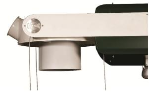
The inlet for type C+S is a standard inlet. The aspiration orifice is 150 mm in diameter, and variable inlet diametres are available, depending on the capacity required. Automatic closing function for negative pressure and false air valves are available as accessories for type S inlets.
