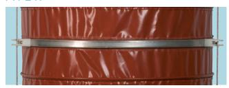
The red module material is Valmex Corotex P250, a rusty-red polyester and fibre glass fabrics coated with silicone rubber on both sides. The type R module has a continuous working temperature area ranging from -40°C and 150°C with short term working temperature on 220°C.
