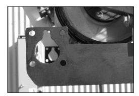
Using the centre point found above and with the mounting plate as a template, trace bolt holes and mainframe hole onto mounting structure. Using a cutting torch or hole saw, cut holes in plate.
