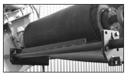
Bolt both mounting plates to the structure. When mounting a single tensioner system, place the tensioner side where it will be the most accessible. Slide the mainframe through the mounting plates and structure so that it is centred on the belt.
