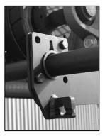
Place the red bushings into the mounting plates with the flange on the outside of the plate. If you are using a single-tensioning system, secure the locking collar on the non-tensioning side, making sure to place it up against the bushing.
