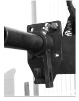
Slide tensioner arm onto the mainframe, with arm facing down and to the right, placing it up against the bushing. Put the adjustment bolt through the bolt pivot, passing it through the oval hole in the mounting plate and through the tensioning arm. The bolt pivot should seat into the radius on the mounting plate.
