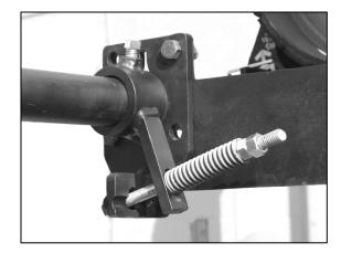
While making sure the blade is contacting the belt, rotate the tensioning arm, forcing the spring up against the nut. Secure it by tightening the two set screws.
