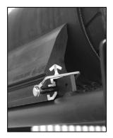
Install the blade onto the mainframe using the supplied pins and centre the blade on the belt.
