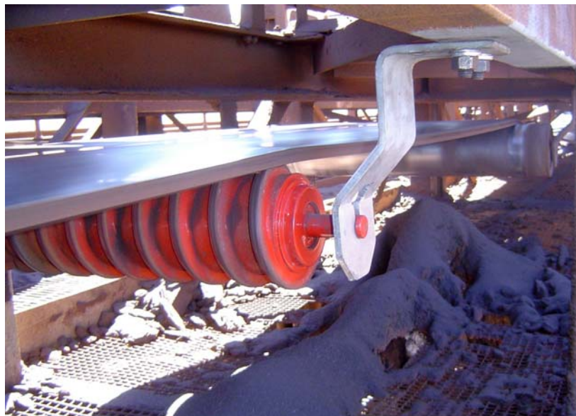
Right: K-Spiromax® Cleaning and Tracking Roller installed on the return belt.
