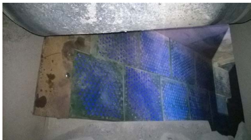
K-Redi-Liner® Ceramic panels showing little signs of wear after 6 months full capacity usage.
