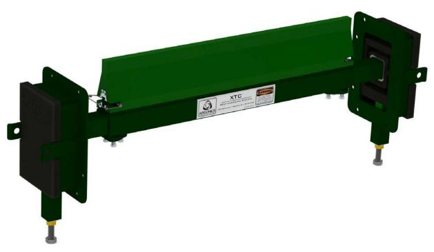
The XTC is a powerful reversing conveyor cleaner. The system can handle wet, dry, sticky or slimy conditions. The unique Web Torque™ tensioner has enough give for mechanical splices and the flow-over blade design reduces material build-up. The XTC is designed with the same toughness and durability as our standard Eraser, with a 6mm thick, 76 mm x 76 mm tube stock steel mainframe and heavyduty stub ends.
