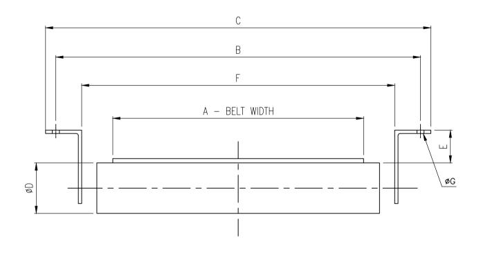
STRINGER FRAME C CHANNEL. ANGLE RHS Is Stringer set up as: TOE IN or TOE OUT TOE IN TOE OUT
