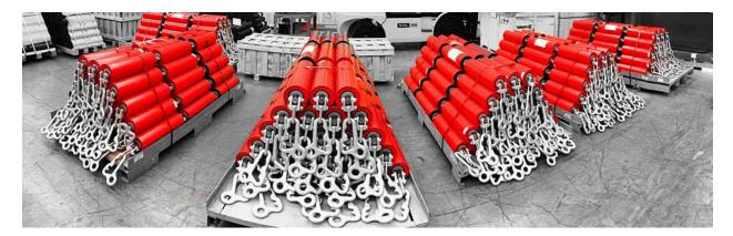
The effectiveness of the K-Steel Roller multilabyrinth nylon low drag sealing system provides an effective barrier to the environmental challenges of dust, dirt, water, low and high temperatures or applications where there is a large temperature gap between day and night.
