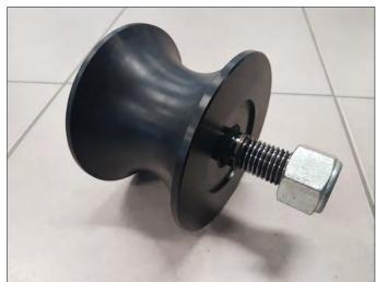
For various reasons conveyor belts wander or mistrack. In other words, guiding does not eliminate the true reason for the belt tracking off centre and it is advisable to examine the root cause of the problem. By examining the cause this may limit the chance of the belt riding over the side guide roller and causing further belt damage.
