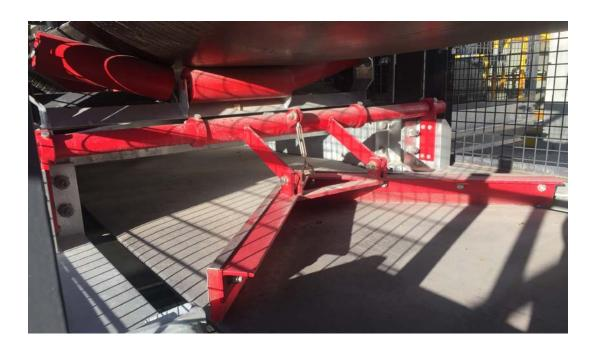
The K-Safeguard Vee Plough Cleaner is a floating return side belt cleaner, suitable for single direction conveyors. This cleaner will significantly reduce spillage and extraneous material from the return side of the belt and is designed to protect the tail pulley. This will aid in belt tracking and reduced maintenance costs and down time.
