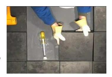
The spacing in between each liner will quickly fill with fine particles that will stay in place creating a solid overall wear surface.
