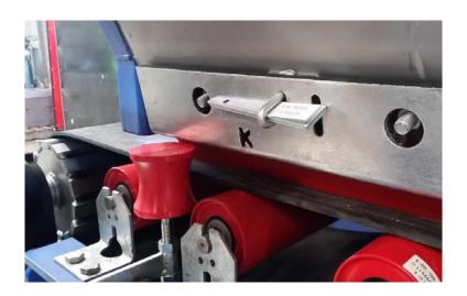
Performing in the same way as the K-Lock<sup>®</sup> Wedge Skirting Clamp, the <u>K-Conlock<sup>®</sup> Clamp</u> <u>System</u> fulfils the practical requirement of a reliable and serviceable system that is free of complications and doesn't rely on the need for special tools to maintain correct seal pressure.
