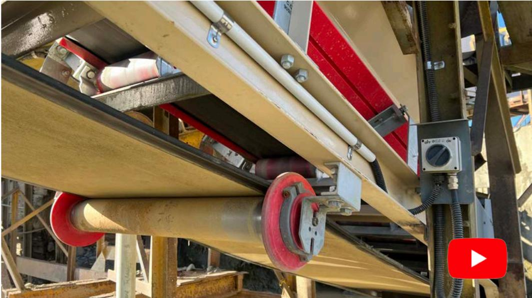
The **K-Commander® Tracking Discs** are a high-performance economical means to track and align a wandering conveyor belt, which is suitable for most installations and bulk materials handling applications.
