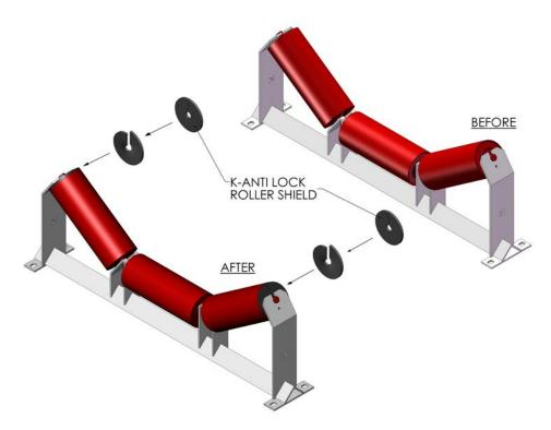
K-Anti Lock Roller Shield is a device which helps to protect conveyor rollers from failure due to seizure. A common cause of belt mistracking which results in material spillage and belt damage is through material becoming jammed between the roller and roller bracket.
