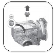
Prior to putting the gearbox into service, the blank plug must be replaced by the breather plug that is supplied with each unit.
