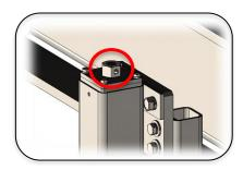
Loosen the take up adjuster locking nuts and raise the cleaner so that the brush bristles just touch the belt. The torque arm bolt will need to be loosened during adjustments.
