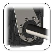
Secure the motor in the desired orientation using the M8 x 20 socket screws. Tighten in a crosswise pattern.
