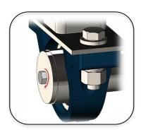
Bolt in the idle side retaining washer and ensure that the shaft is positioned so that the bearing is contacting the washer. Fully tighten the grub screws.
