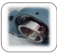
Tighten the grub screws on the bearings with the 5mm hex key so that they do not move around during installation.
