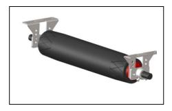
Above: Image of the Tru-Trac® Conveyor Belt Tracking System - the range covers self-aligning idlers for tracking both the return and loadcarrying sides on slow moving, reversible, high-speed and high-load belts up to 2500mm.
