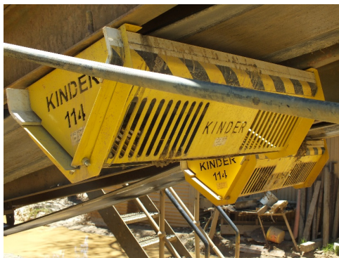
Close-up photo of the K-Protector® Return Idler Guard installed on one of the return rollers
