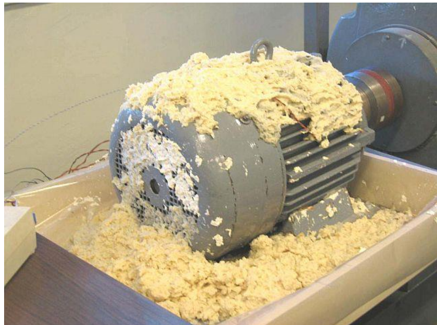
Set in a laboratory, photo example of pulp clogging the motor
