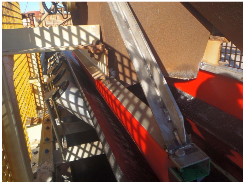
Above: Installation drawing for K-Snap-Loc Dust Seal System showing weld point and retaining pin Right: Close-up image of conveyor chute and K-Snap-Loc after installation.
