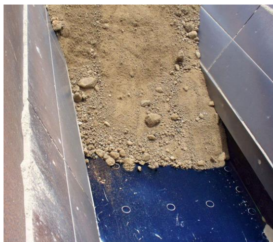
Right: a typical example of K-Superline installed in a chute.
